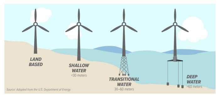
Offshore wind turbines may be built in shallow waters, anchored in the sea floor, or floating in deeper waters. Though they can be constructed nearshore, most turbines are miles offshore and barely visible from shore.
